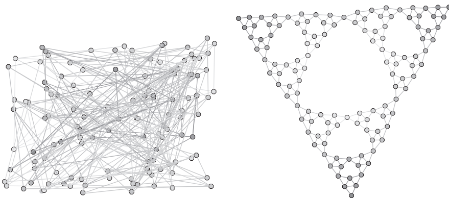
FIGURE 14.3 A random drawing of a graph and a drawing of the same graph produced by a force-directed algorithm.
